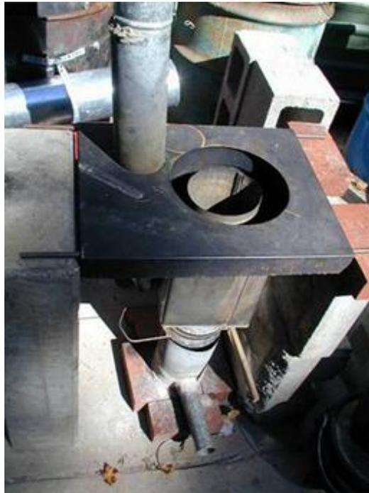
Photos of the original Champion stove that won the clean combustion contest in 2005. This unit was built in Cochabamba, Bolivia, for operation at over 2000 meters elevation.
