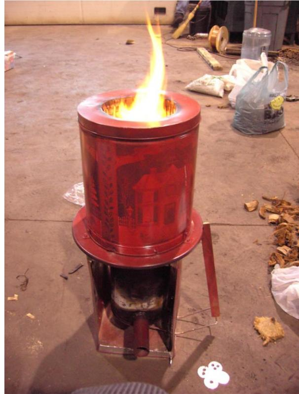
The disk in the bottom rises under the fuel canister, and is held in the raised position by the red stick on the outside. Note the metal controller of the primary flow.
