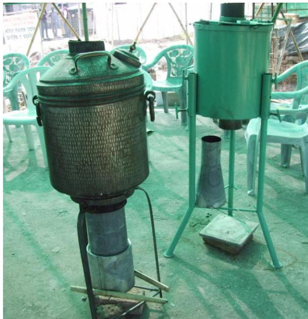
TLUD stoves made in India. Note the sliding connectors. Several are for water heating.
